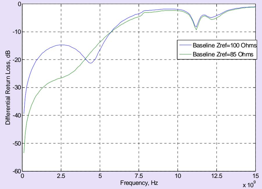
The standard thru-hole PCIe connector has very reasonable performance for 8 GT/s. There *might* be a need for better connectors for topologies with long routes and thick PCB
