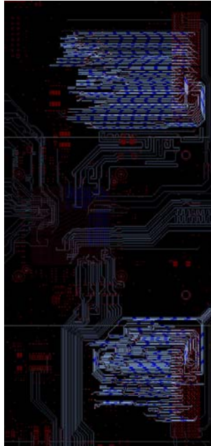
Figure 4-8. Processor Interface Bus A and B In and Out, Layer S07
