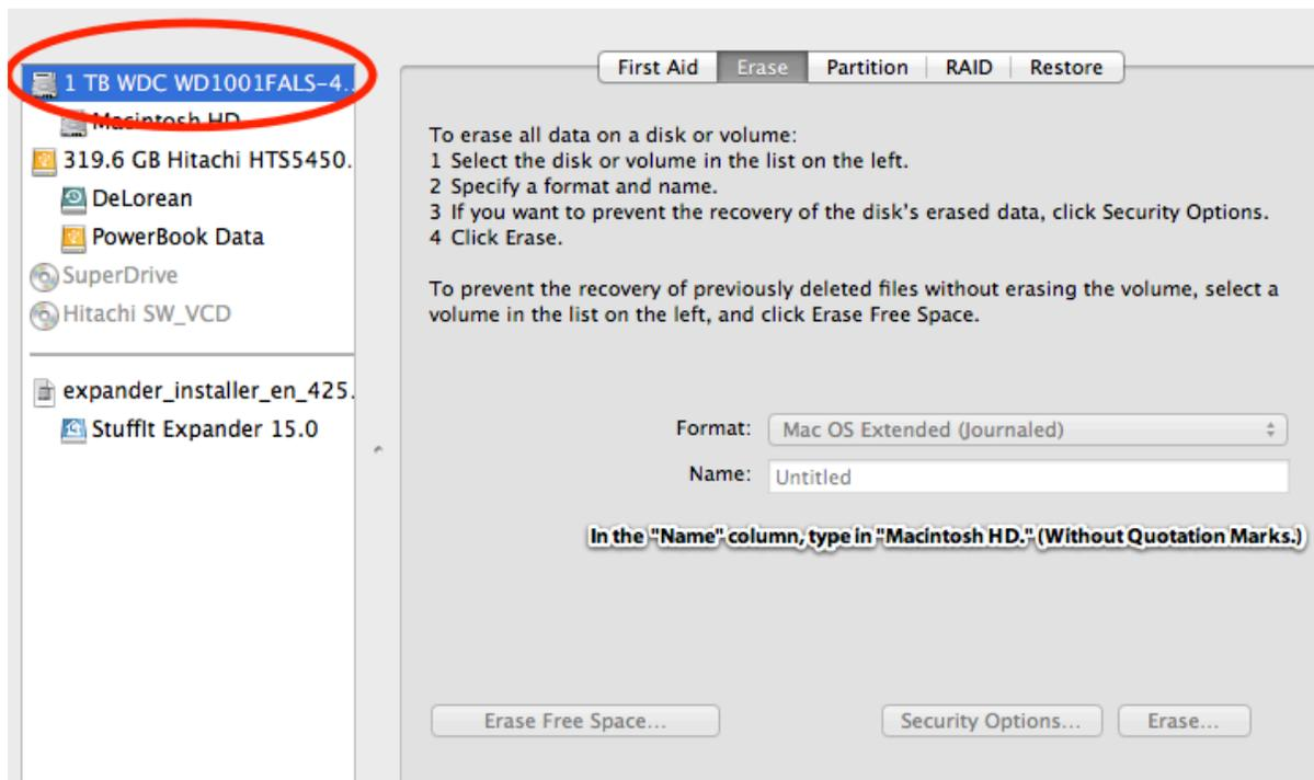
Example: Your Mac has a 1 terabyte Western Digital hard drive. Disk Utility would list it as a "1TB WDC" drive, with the model number following. Select the "1TB WDC" entry, and click the erase tab. You are now at the proper tab to erase your drive.
