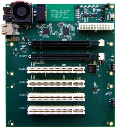
Figure 1: PCI / PCIe Expansion Backplane
