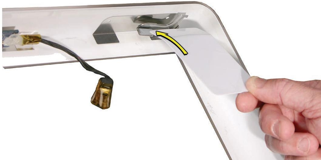
5. Start on the left side (looking from the back of the unit). As you insert the card to disengage the latch, squeeze the top of the bezel, that will help take pressure off of the latch and enable it to open easier. As the bezel releases, pull the bezel away from the rear housing. Note: If the bezel won't open, try cutting the card lengthwise into 3/4 inch or 1.5 cm strips. Insert the card again, on a 45° angle, aimed toward the outer corner, and try again.
