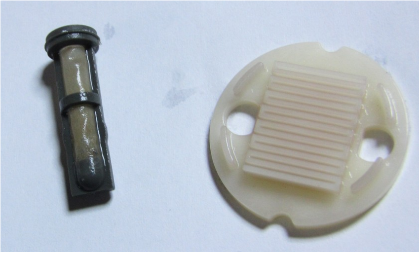
Screen filter and white maze of a CPU block
