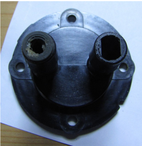
CPU block top showing some residue
