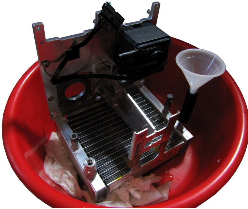
Setup for radiator cleaning with vinegar
