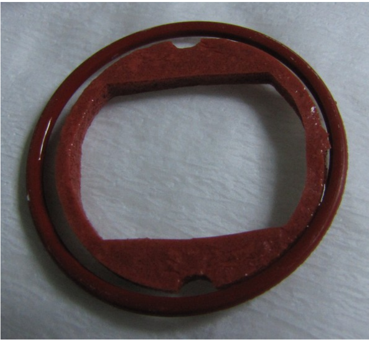
CPU block O-ring and red foamy pad
